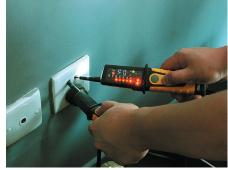
A must for all service people. This instrument indicates the presence of AC/DC Voltage and displays the voltage levels. It is easy to carry, light weight and completely fool proof.
