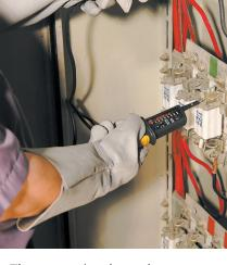
The most simple and easy to use voltage detector that is a must for all technicians. Not only does it measures and dectects voltage, it also determines phase rotation directions.
