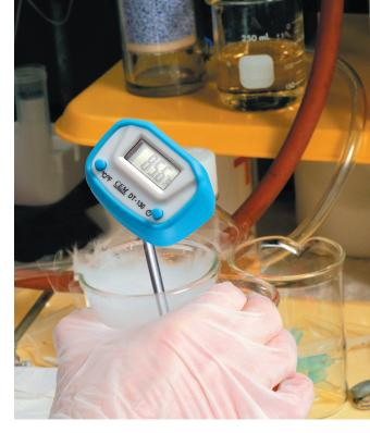
This contact type thermometer offers fast response and laboratory grade accuracy. This meter offers 0.1°C/0.1°F resolution over the entire measurement range. A rugged holster protects this model.
