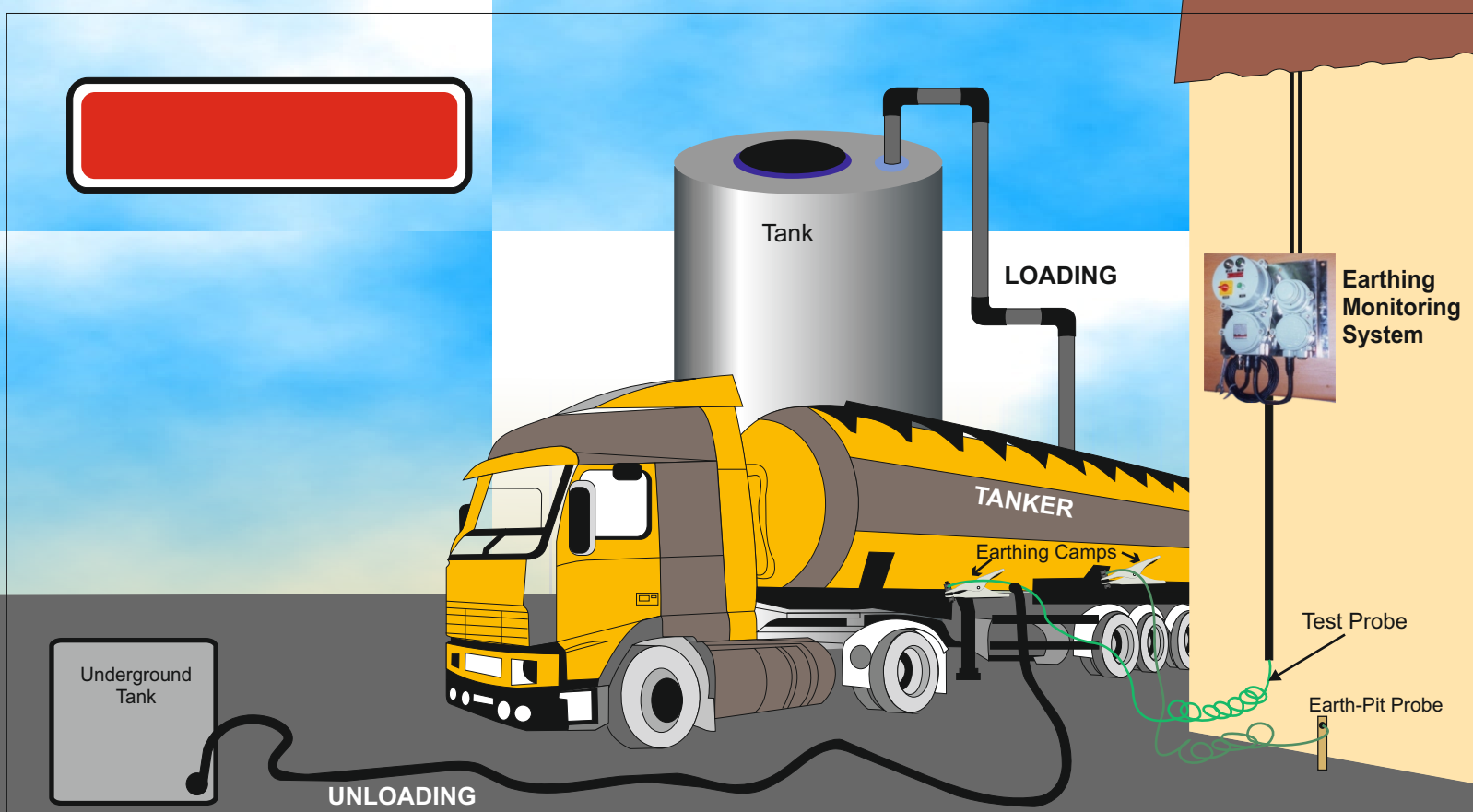
FLAMEPROOF TANKER LOADING UNLOADING EARTHING SYSTEM
