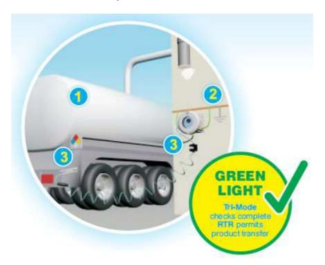
1) Road Tanker Recognition: As soon as the operator applies clamp of RTR System on the road tanker (immediately when tanker visit tank farm area) it will check that the clamp is applied on tanker by checking tanker's capacitance with respect to earth. If by mistake operator applies this clamp on any other earthed structure than first check will not get ok then system will not become permissible for second check.
